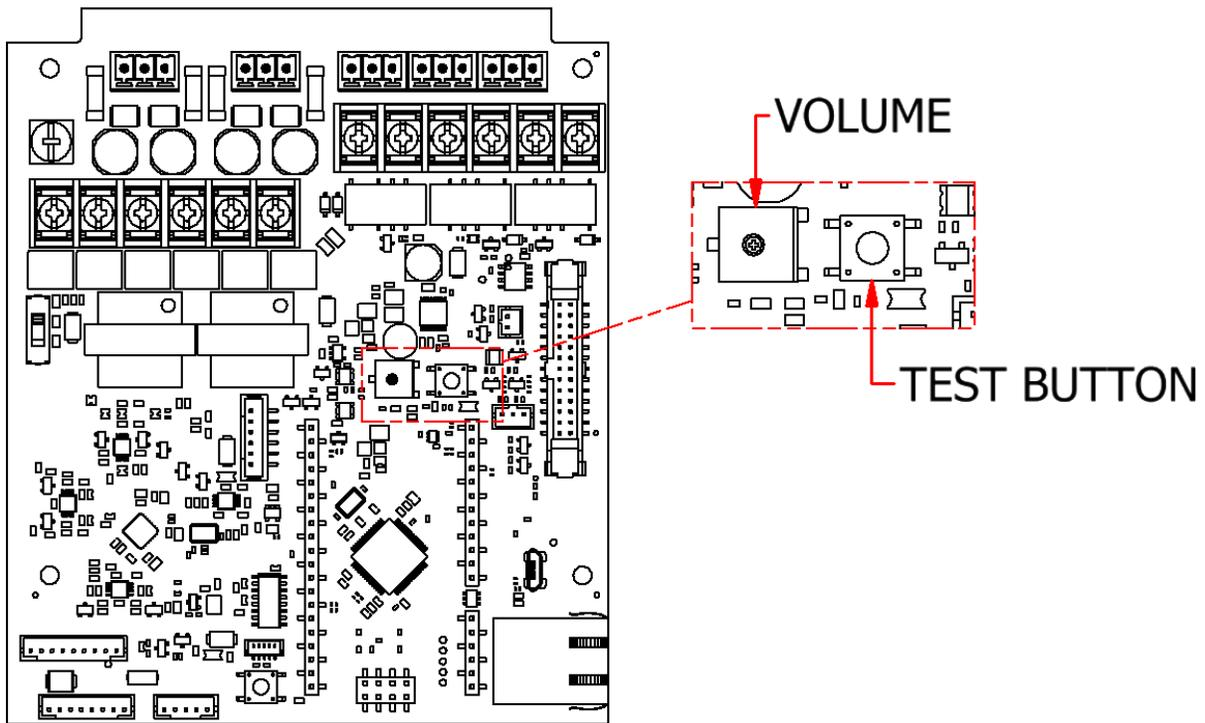
Figure 20: Test Button and Volume Adjustment
