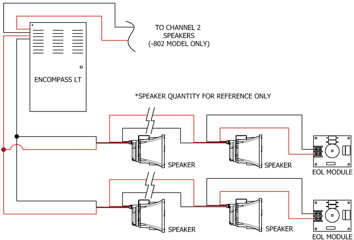
**Figure 8: Speaker Wiring**
