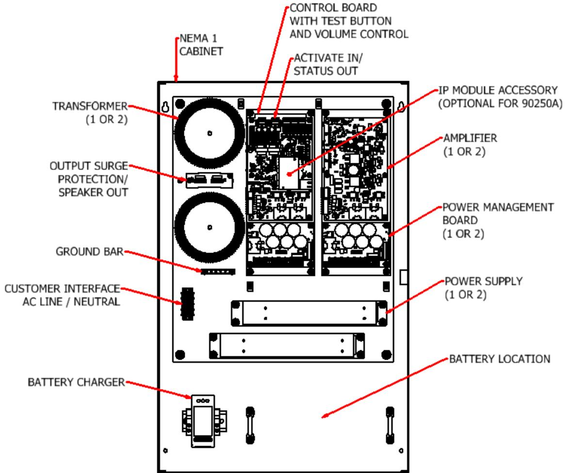
Figure 3: -802 Internal Cabinet Detail
