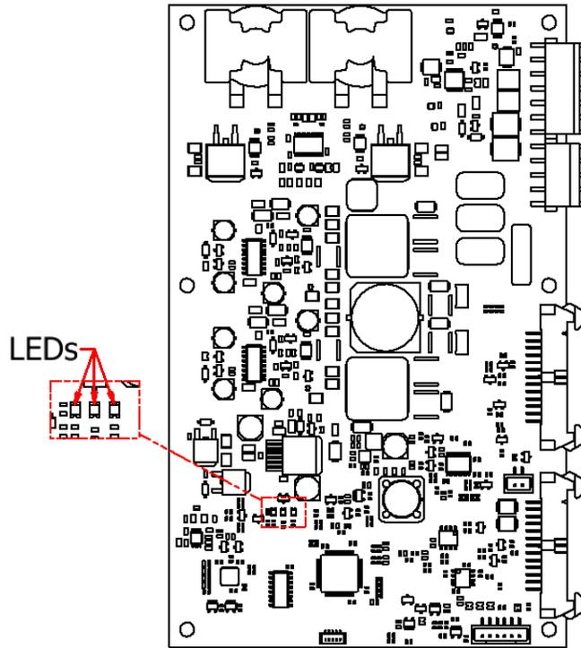
Figure 22: Amplifier Status LEDs
