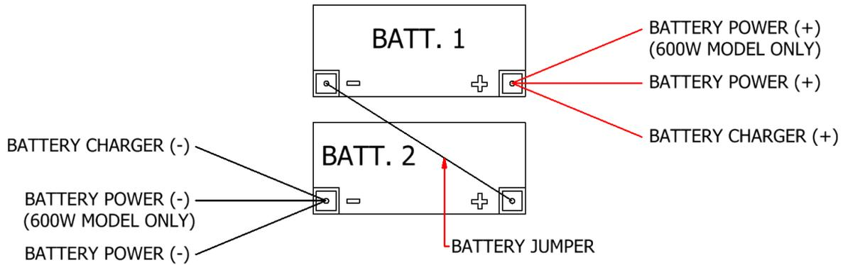
Figure 16: Battery Connections
